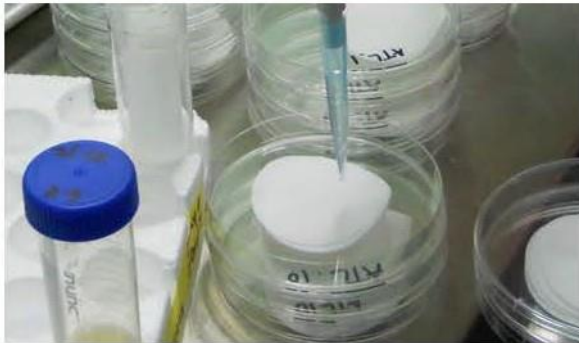
Left: Carriers being Inoculated with Test Microorganism
